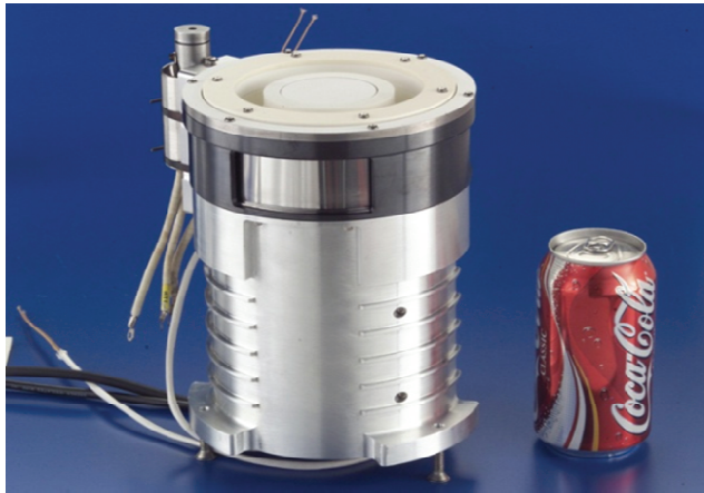
Fig. 6. HiVHAC laboratory model thruster.
