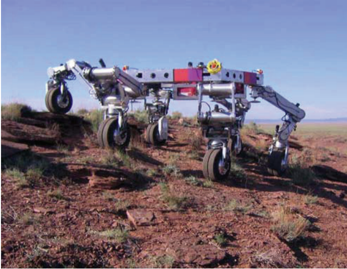
Fig. 14. Wheel-leg Hybrid system ATHLETE (Image Courtesy: NASA/JPL/Caltech)
