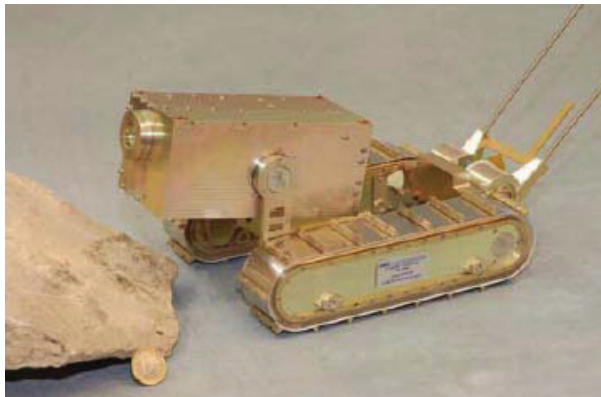
Fig. 6. Nanokhod dual-track system (Image Courtesy: Klinker, 2007)
