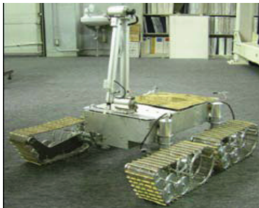
Fig. 8. JAXA’s four track system (Image Courtesy: Wakabayashi, 2006)
