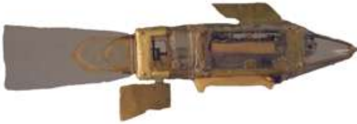
Figure 1.4: “Artificial fish” built by Miles Pebody to explore influence of robot bodies on behaviour. The fish could swim around by wagging its tail and avoid obstacles based on infrared sensing.
