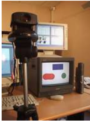
Figure 1.2: A single “Talking Head”. There is a camera oriented towards a white board. The bottom screen shows what the camera observes. The top right screen shows the result of processing. A loudspeaker reproduces the utterances of the agent.
