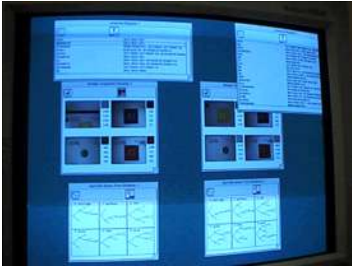
Figure 2.2: Interface through which the internal states of agents can be inspected. Two agents are shown. The top windows show the state of an agent, the middle windows the camera inputs that the agent sees and the bottom windows show their discrimination trees.
