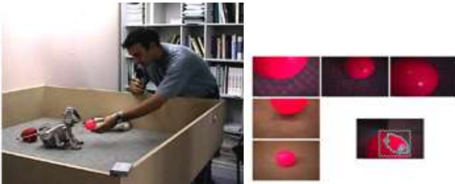
Figure 10.1: Left: Frédéric Kaplan interacts with the AIBO robot in an experiment for the social learning of lexicons. Right: View of the ball through the eye of the robot. As the same object is now seen from many different viewpoints it becomes much more challenging to consistently recognise it.
