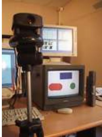
Figure 8.3: A single Talking Head at the Paris site. In the background we see (bottom) the display with an image that the agent picked up, (on top of that) a screen displaying the processed image and the discrimination trees, and to the right the loudspeaker broadcasting the speech output of the agent.
